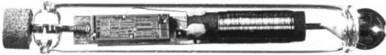
Fig. 1. Microstimulator, from left: anodized Tantalum (Ta)-slug, hermetic seal to glass bead and glass capillary walls, Ta stem welded to gold plated metal shim, integrated circuit (IC) chip with Au wirebonds to copper (Cu) coil, Ag-epoxy junctions to Cu coil windings over hollow ferrite core, Ag-epoxy connection to iridium (Ir) ball sealed to glass capillary wall, activated Ir surface.
