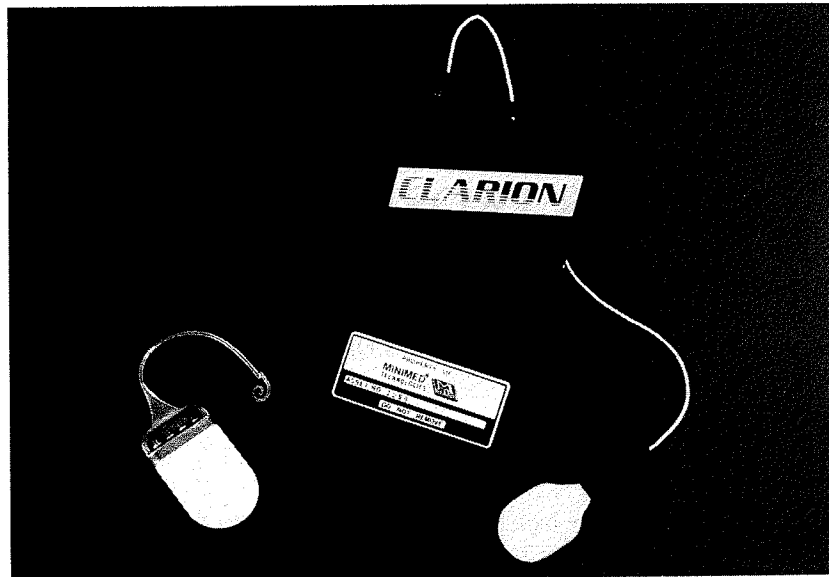
Figure 1 Clarion™ cochlear prosthesis produced by Minimed Corp. of Sylmar, California, showing spirally molded electrode and ceramic case (lower left) containing custom IC chip and related circuitry for driving the 16-contact electrode array with signals specified by the external speech processor unit (center) and transmitted along with power by an inductive coil (bottom right). (Photograph courtesy of Minimed Technologies.)
