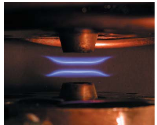
Researchers are studying how gravity influences the combustion of solid fuels using this opposed jet flame configuration.
