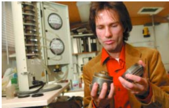
Constantinos Sioutas sets up an air concentrator to measure tiny particles of urban pollution.
